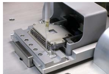
Pipetting robot and wash probes in action.
