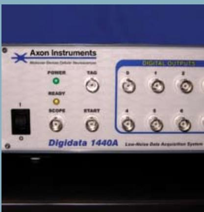
Digidata 1440A offers front-panel access to digital triggering, tagging, and output BNCs.
