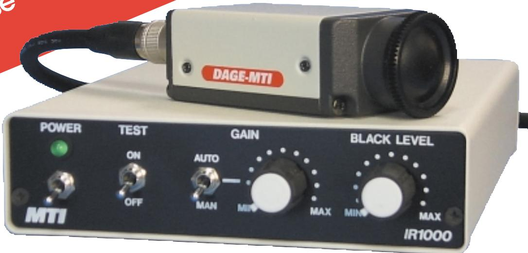
The IR-1000 infrared CCD camera is designed especially for applications requiring high sensitivity in the near infrared. The high gain of the camera enables the user to detect images in real-time (30 frames/sec.) even when energy levels are very low. With wide range gain and black level controls, the IR-1000 enables the user to enhance image contrast and offers the ability to do short-term integration for increased sensitivity.
