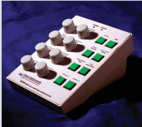
To offer a more conventional amplifier control, the optional SoftPanel was designed as a hardware extension of the Axoclamp Commander software. SoftPanel communicates with the computer via an easy-to-set-up USB 2.0 connection. Using SoftPanel does not negate the many benefits afforded by computer control of the amplifier.
