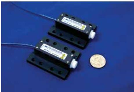
The small profile of the miniaturized HS-9A and VG-9A headstages makes it easy to incorporate them into an electrophysiology set up. The dovetail design integrates with a baseplate for easy attachment to micromanipulators.
