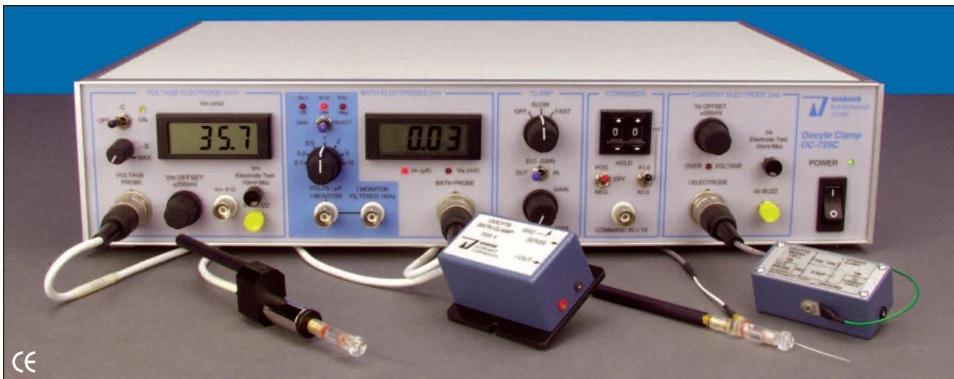
The **OC-725C** Oocyte Clamp is designed for two-electrode, whole-cell voltage clamping of *Xenopus* oocytes. The dedicated design of the OC-725C includes such features as high compliance voltage ( $\pm 180$  V) and unique bath clamp circuitry. These same features also make the OC-725C ideal for clamping other large cells and cell structures such as squid axons. Improvements to this version include an extended current measuring range, decreased noise level and a 4-pole Bessel filter.
