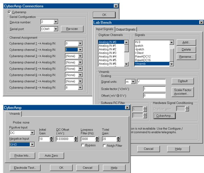
CyberAmp control is built into Clampex 9 and into AxoScope 9. Assigning a CyberAmp channel to an analog input automatically enters the CyberAmp gain in the software scaling of that input channel, and stores the CyberAmp filter settings in the recorded data file.
